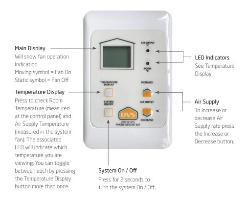
Turning the system **ON** or **OFF**: Pressing the SYSTEM ON / OFF button for 2 seconds will turn the system off (display and LED's off, fans off). Another press will turn the system back on.
