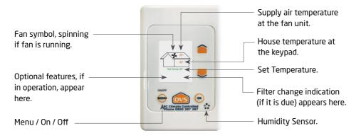
**Turning the system ON or OFF:** Press and hold **MENU** to turn the system On or Off.
